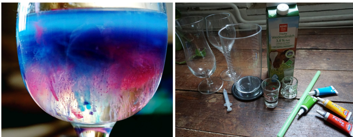
Figure 2. Cloud tank experiment (left) and the necessary utensils (right): actually used as a visual effect in movies to simulate clouds, it was used as an experiment on PW-tours to show density differences of fresh and salt water to explain how ocean currents are driven by density differences.
